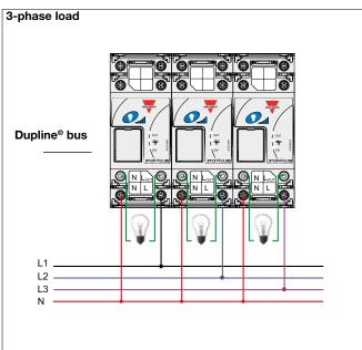
Note: The cable between the dimmer module and the light should not exceed 25 metres
